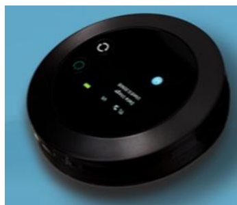
Figure 2-13: Virtual SIM example: TEP Wireless Pocket WiFi device
