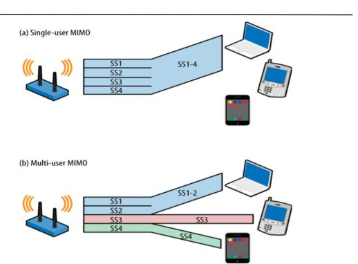
Figure B 4: Single-user MIMO vs. Multi-user MIMO
