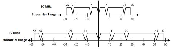
Comparison between 20 MHz and 40 MHz channels in WiFi 4
