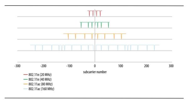
Figure B 6: WIFI 4 Channels Vs. WiFi 5 Channels
