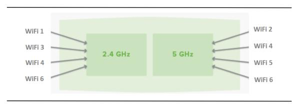
Figure B 7: Operating frequencies in different WiFi generations
