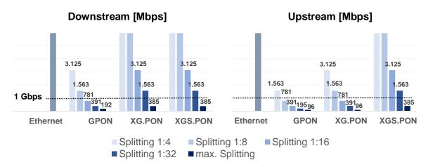
Source: WIK. The maximal splitting ratio is set at 1:1 for Ethernet PtP, 1:64 for GPON and at 1:128 for XG.PON and XGS.PON.
