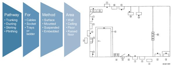
Figure 4-14: Overview of cable trunking and ducting systems
