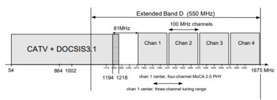
Figure 4-7: MoCA 2.5 extended band D frequency plan
